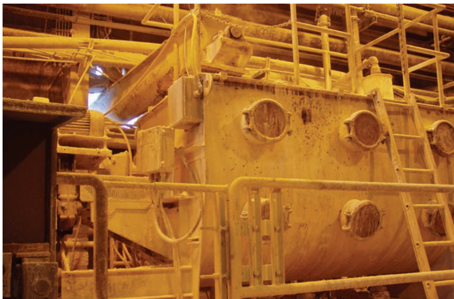
U-shaped lime slakers mix water and dry lime together to create milk of lime, which is used to raise the gold slurry’s pH level during the neutralization process.
