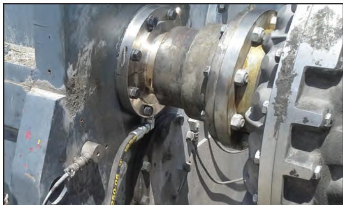
An external drain was designed to accommodate the operational flood in the Sag Mill Gearbox bearing housing.
