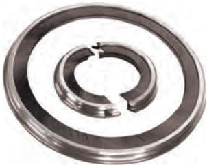
The Sentinel FBS is a drop-in replacement for a standard carbon ring seal. The brush serves as the primary shaft seal while a carbon element provides face sealing in the turbine's casing. Users have found that by utilizing the FBS, the interval between seal replacement increased more than 3x to an average 3 to 4 year life span.
